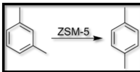
Fig5. Isomerisation of meta-xylene to para-xylene on passing through a ZSM-5 catalyst.
