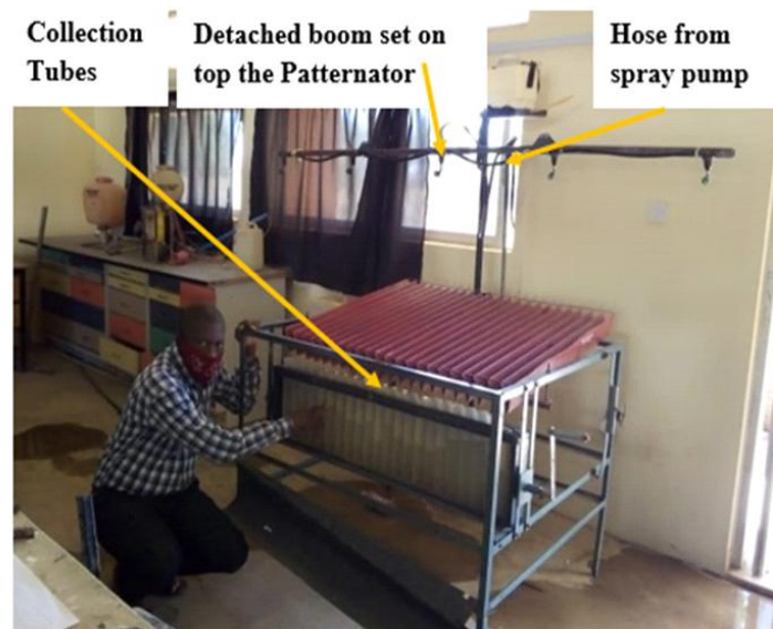
Plate II: Patternator test rig inside the laboratory. The detached boom is mounted on the test rig
