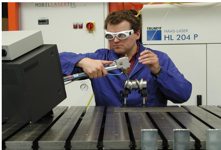
Fig. 1 The process of manual laser surfacing of shafts with the addition of a laying wire by hand, using a video monitoring system for the process [1].
