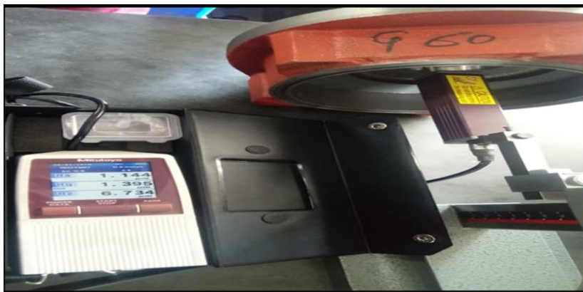
Figure 10: Mitutoyo Surface Roughness Tester used for surface roughness measurement
