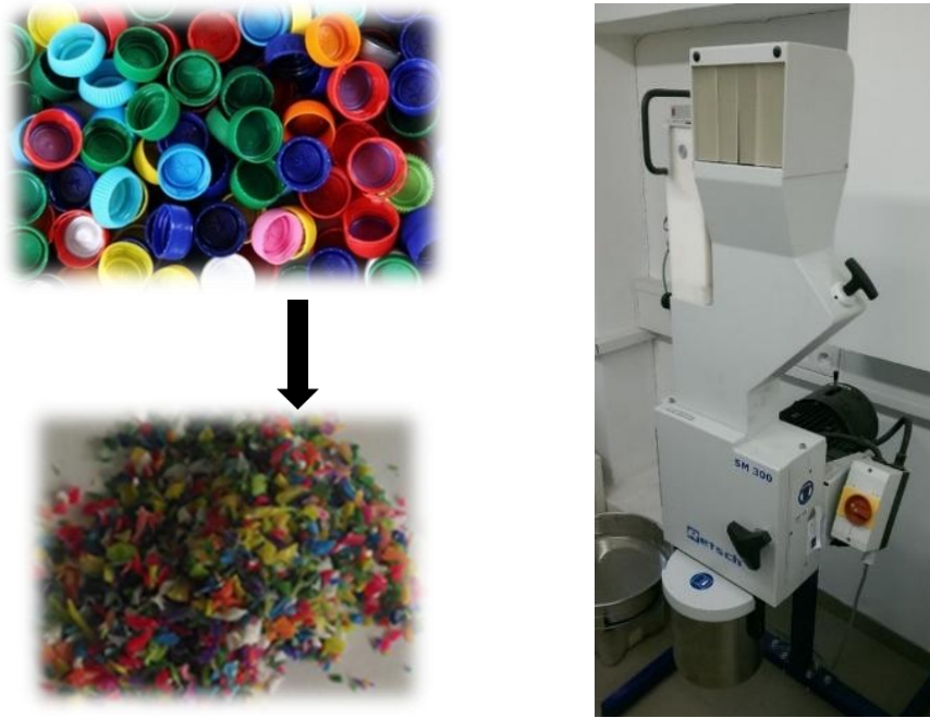
Fig. 1 Disintegration of PET bottles and Retsch cutting mill
