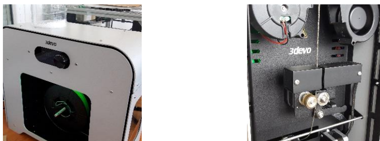
Fig. 2 Filament Maker Composer 3devo
