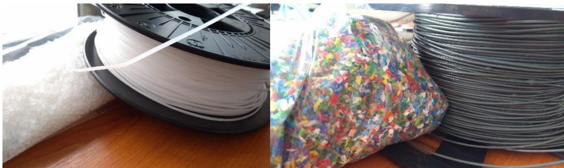
Fig. 3 Filament produced from waste based HDPE 1 Fig. 4 Filament produced from waste based HDPE 2
