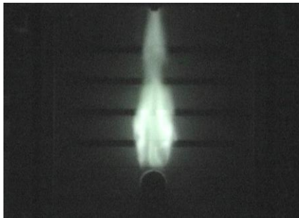
(C3) Lift-off flame ( U_{in}=1.39\text{m/sec} ) (Night shot photograph)
