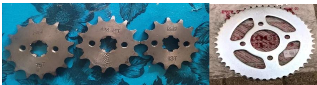
(a) (b) Figure 1. Sprocket gear a) front sprocket gear b) rear sprocket gear
