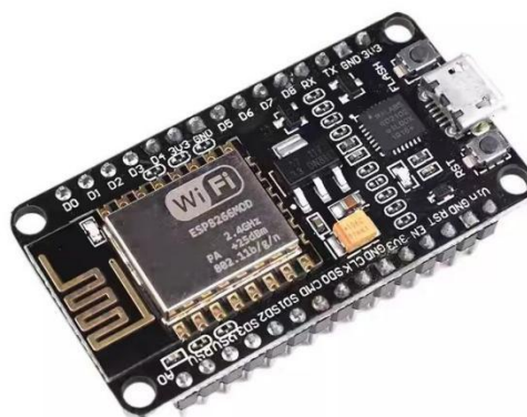
Fig. 5 EPS8266WiFi Serial Port Module
