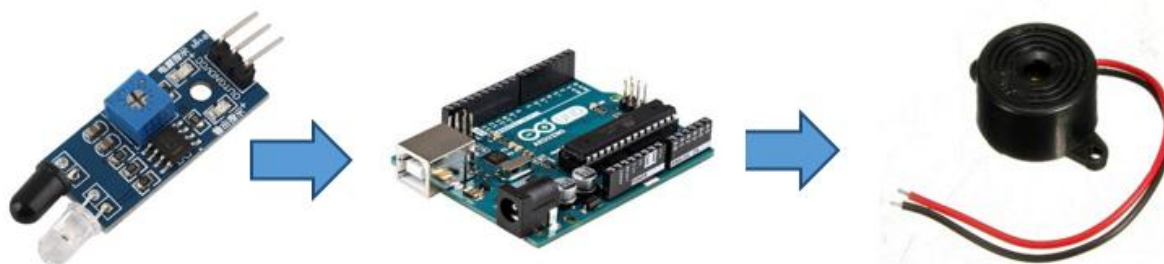
Fig. 4 Home security automation technical design
