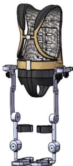
Fig. 1 Schematic diagram of the overall structure of the lower limb exoskeleton device
