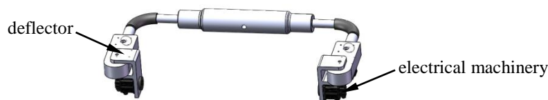
Fig. 2 Schematic diagram of lower extremity exoskeleton hip joints
