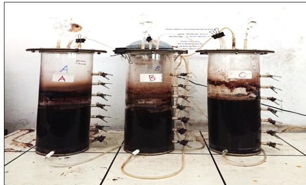
Fig. 3 Anaerobic circular batch reactor on a laboratory scale (CBR)
