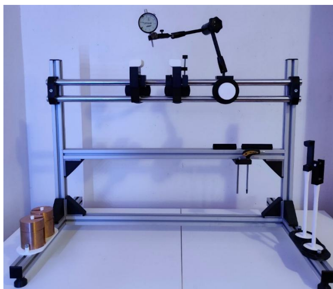
Fig. 5 In-house device for bending and torsion testing of polymer materials
