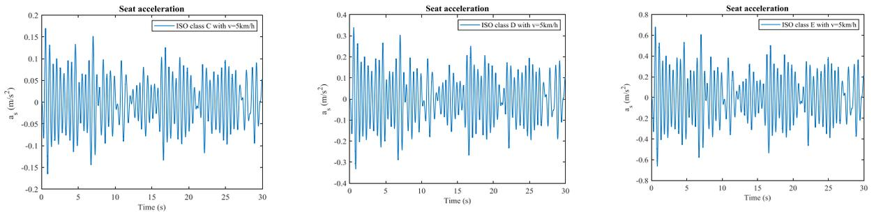
**Fig.2.** Driver’s seat acceleration under three poor road surface conditions at v=5km/h and full load
