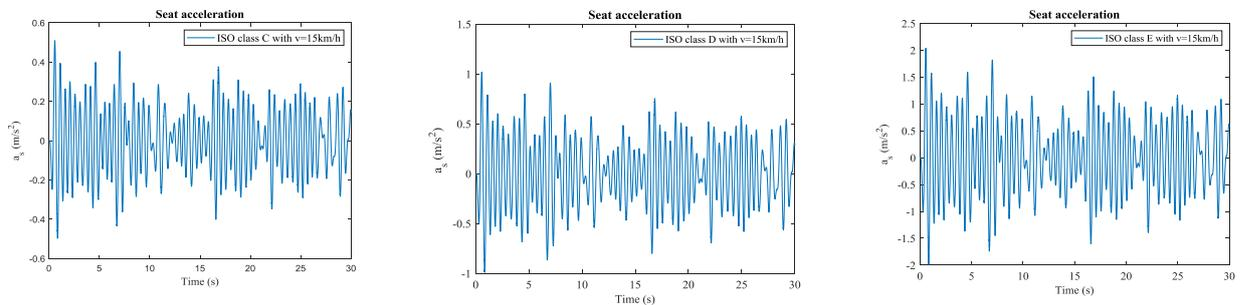
**Fig.4.** Driver’s seat acceleration under three poor road surface conditions with v=15km/h and full load
