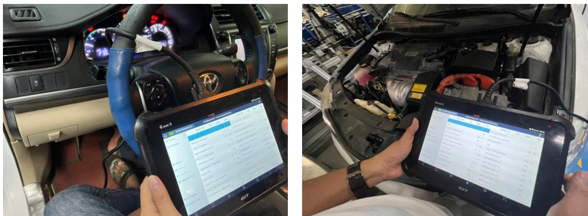
Figure 1. Students performing diagnostic exercises on a Toyota Hybrid vehicle using the G-scan 3 diagnostic scanner
