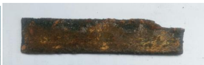
Fig. 10.0, Group A. Corrosion Test Specimens, (Mild Steels And Copper) After 480Hours Exposure In 0.5Mol. Aqueous H_2SO_4 .
