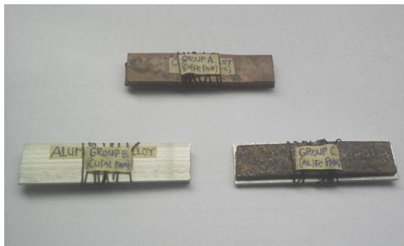
Fig. 2.0, Dimensioned Metallic Specimens, (Mild Steels, Aluminium Alloys, And Copper Alloys),
