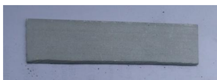
Fig. 12.0, Group C. Corrosion Test Specimens, (Aluminium And Mild Steel) After 480Hours Exposure In 0.5Mol. Aqueous H_2SO_4 .
