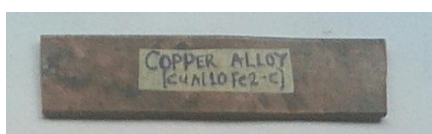
Fig. 10.0, Group A. Corrosion Test Specimens, (Mild Steels And Copper) After 480Hours Exposure In 0.5Mol. Aqueous H_2SO_4 .
