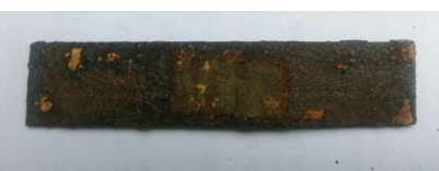
Fig. 12.0, Group C. Corrosion Test Specimens, (Aluminium And Mild Steel) After 480Hours Exposure In 0.5Mol. Aqueous H_2SO_4 .
