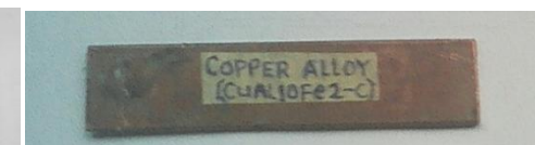
Fig. 11.0, Group B. Corrosion Test Specimens, (Copper And Aluminium) After 480Hours Exposure In 0.5Mol. Aqueous H_2SO_4 .
