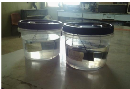
Fig. 8.0, Paired Test Coupons, Immersed In 0.5 Mol. Concentration Of H_2SO_{4(aq)} Electrolyte After 120Hrs,
