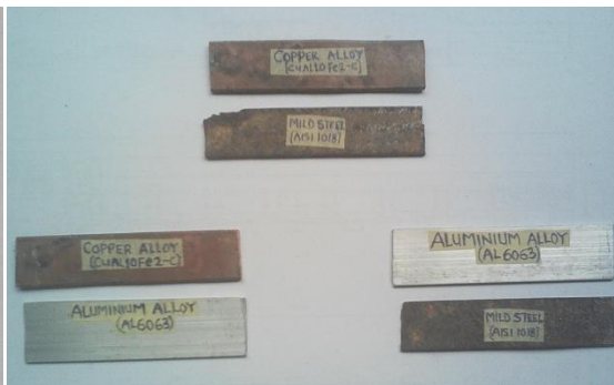
Fig. 3.0, Pairs Of Corrosion Test Coupons, (Cu/Fe, Cu/Al, And Al/Fe).
