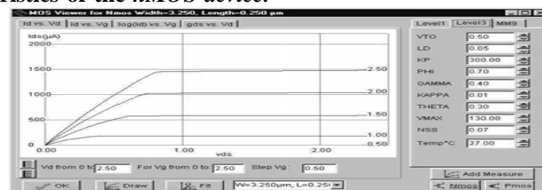
Fig. 21(b): N-Channel MOS characteristics.
