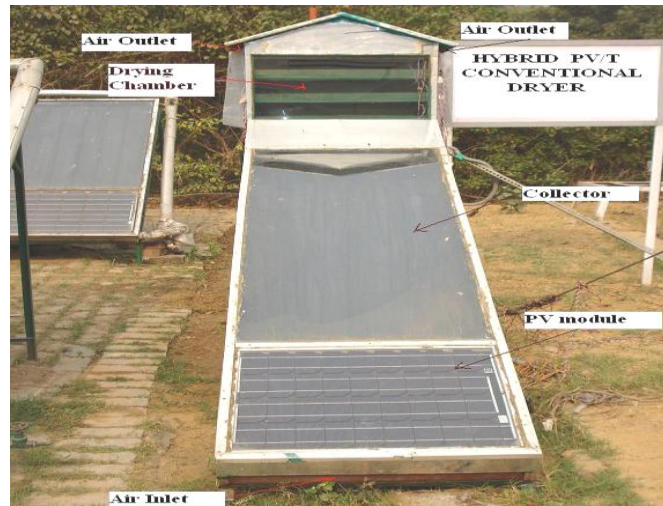
Figure 1: Photograph of hybrid Photovoltaic-thermal (PV-T) integrated solar dryer
