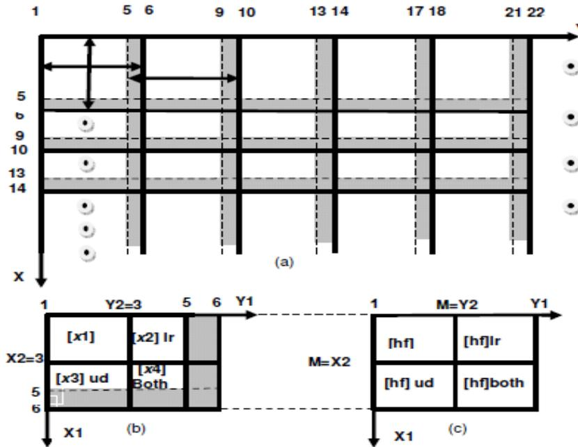
fig 1: Layout of the Partitioning grid for the input Image Filtering pass.
