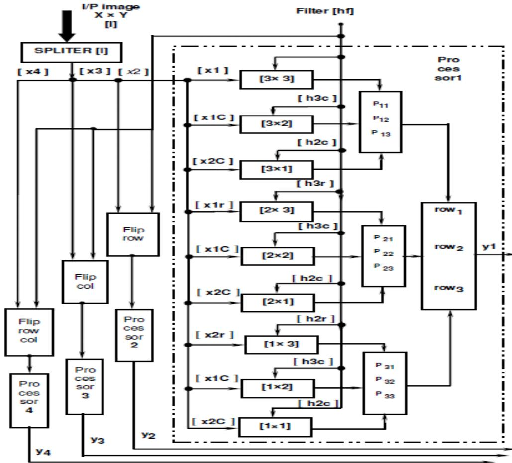
Fig 2: Algorithm for small Convolution
