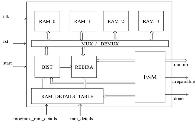
Fig 3.1: Block diagram of the proposed Re-BISR scheme for repairing multiple RAMs
