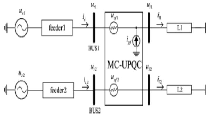
Fig. 1. Single-line diagram of a distribution system with an MC-UPQC.
