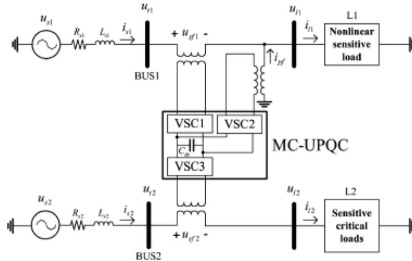
Fig. 2. Typical MC-UPQC used in a distribution system.
