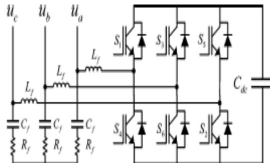
Fig. 3. Schematic structure of a VSC.
