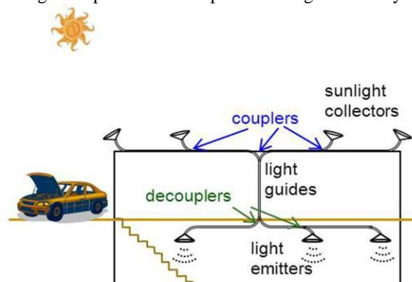
Fig. 1. Schematic of a daylighting system with a building layout.
