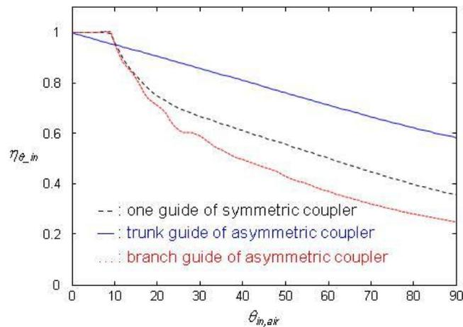
(a) Accumulated coupling efficiency of individual light guides.
