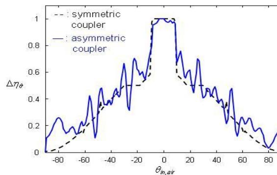
(c) Total angular coupling efficiency ( $\theta_{coup} = 40^\circ$ )
