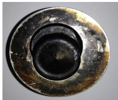
Figure 4. Shallow Torodial piston
