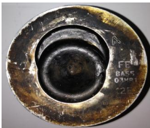
Figure 3. Deep Torodial piston
