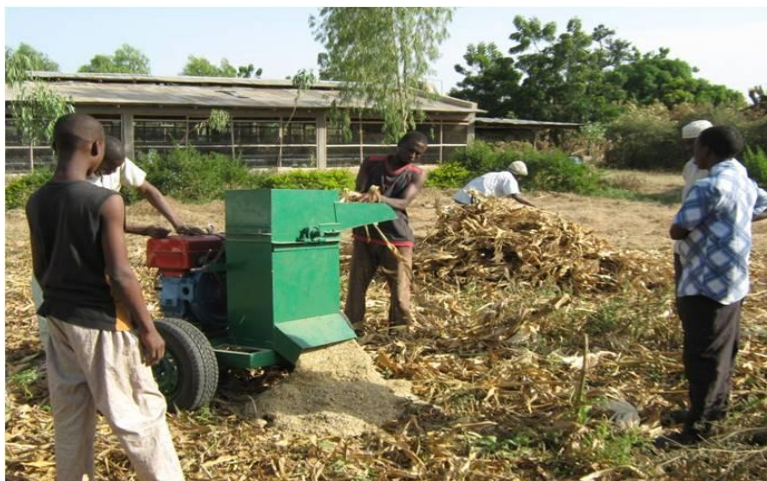
Fig. 3 shows the fabricated machine in operation while the crushed residue is discharged.
