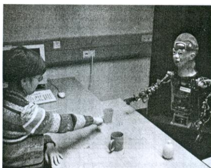
Fig. Using deictic gestures to show and teach BARTHOC junior new objects
